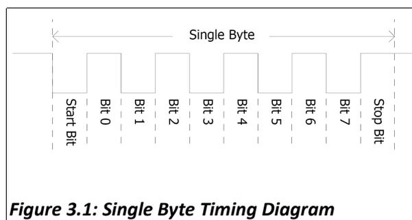
Figure 3.1: Single Byte Timing Diagram
